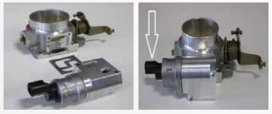
Using the new gasket and hardware supplied in the kit assemble the IAC valve and adapter to the BBK Throttle Body.
