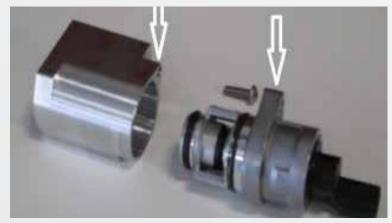
To install the IAC value into the supplied adapter. Line up the bolt holes and press the IAC value into the adapter supplied in the kit. Using the supplied bolt tighten it down to secure the two pieces together.
